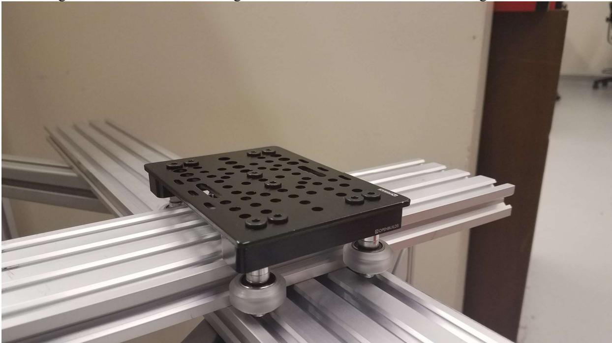
Figure 4 X-Axis Carriage Assembly
