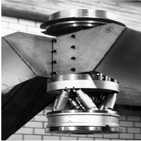
Figure 2.10 Application of parallel robots
